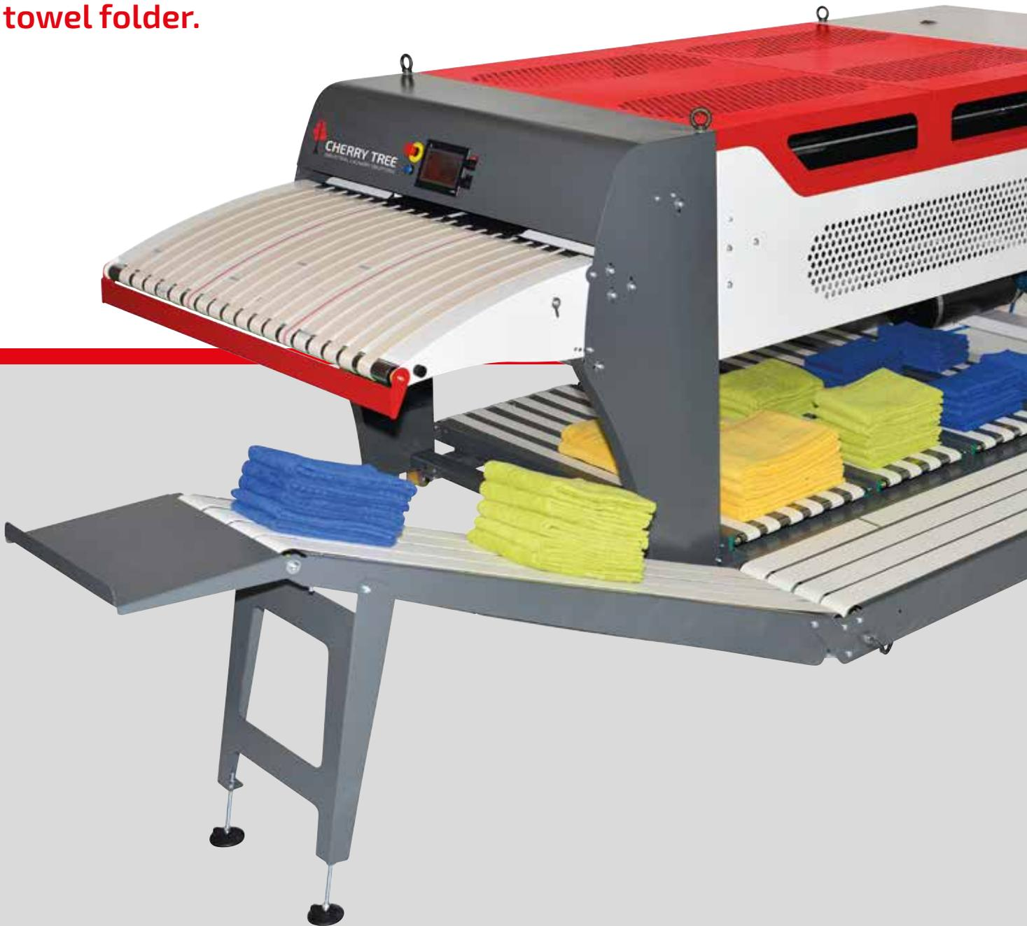
The new powerful feeding conveyor can be adapted in height to make it suitable for short and long operators. The conveyor has been extended, resulting in a better grip for longer towels.
